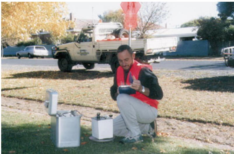
Gravity survey by contractors, Geoterrex, in street environs, in the REDAN area of Ballarat West in 1997, with permission of the former Ballarat Consolidated Gold Ltd.
