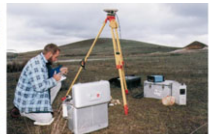
Lone Hand No.2 Base Station. Daily readings, gravity survey Geoterrex crew 1997 working on EL 3821, Allendale
